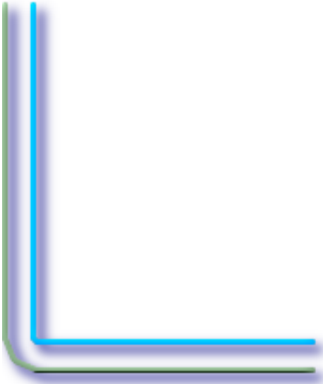
15, 'quad_segs=4 join=bevel' shown with original line
