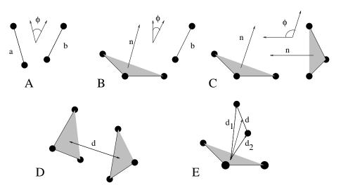
Figure 8.6: Options of g\_sgangle: A. Angle between 2 vectors. B. Angle between a vector and the normal of a plane. C. Angle between two planes. D. Distance between the geometrical centers of 2 planes. E. Distances between a vector and the center of a plane.
