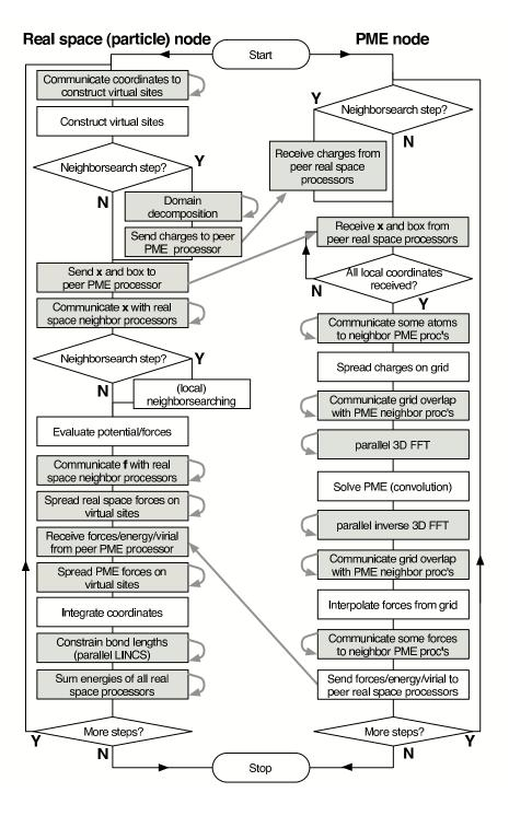
Figure 3.15: Flow chart showing the algorithms and communication (arrows) for a standard MD simulation with virtual sites, constraints and separate PME-mesh nodes.
