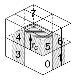
Figure 3.11: A non-staggered domain decomposition grid of  $3 \times 2 \times 2$  cells. Coordinates in zones 1 to 7 are communicated to the corner cell that has its home particles in zone 0.  $r_c$  is the cut-off radius.
